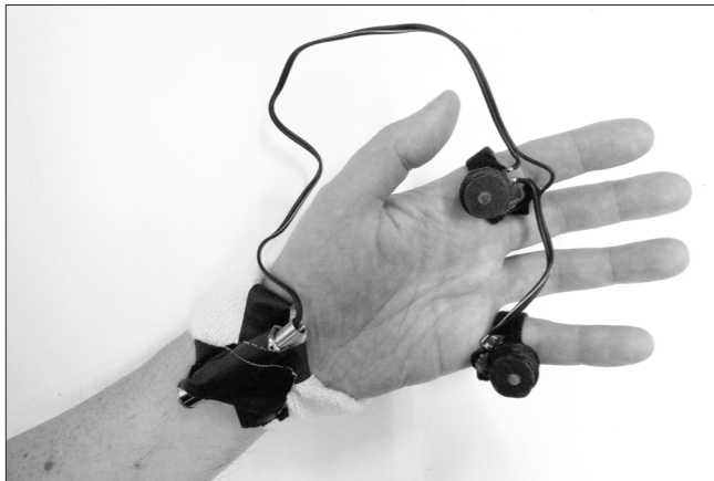
custom built magnetic pickup
